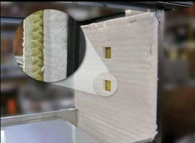
**Better lifetime performance** - Hybrid insulation with a layer of Superwool® HT for improved insulative qualities.
